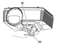
6. Remove the tape fixing the lamp replacement attachment, and remove the lamp replacement attachment with the lamp unit remaining in the bag.
